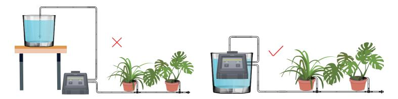
2.2 The lift length of the water pump: the vertical distance of 2-3m, because the water pipe can not be placed 100% straight, we recommend that the height of the plants than the pump should not exceed 2.5m.
