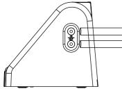
3.3 Connect the hose to water inlet and outlet
