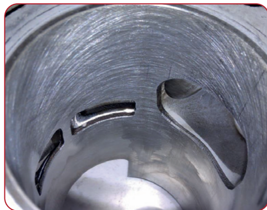
PIC 1: PROPER PORT CHAMFERING ALLOWS SMOOTH TRANSITION OF THE RING DURING TRAVEL
