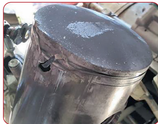
PIC 2: EROSION OF THE PISTON FROM DETONATION WILL ANNEAL THE PISTON MATERIAL, CAUSING FAILURE
