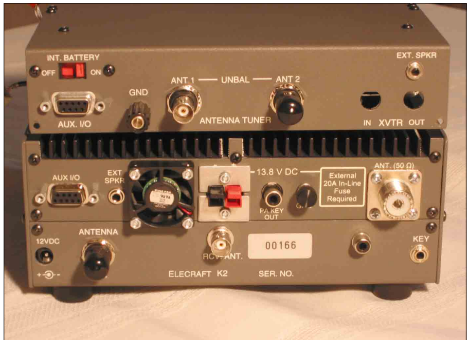
Figure 3—Rear view of the 100 W K2
