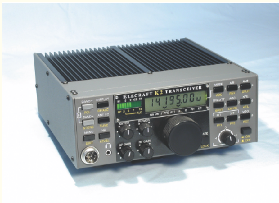
The Elecraft K2/100, a 100 watt HF rig you can build yourself.
