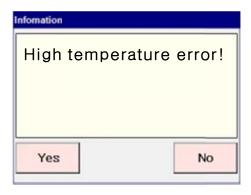
Solution →Check temp. setting / Replace thermocouple.
