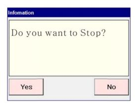
Solution  $\to$  To stop the cycle press the "Yes" button. The oven will continue operation after 5 seconds if no buttons are pressed.
