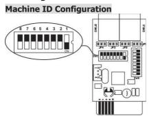
There are eight bits to present ID of each card. Use SW1 to set machine ID. There are eight bits. From left to right, it's 8 to 1. As shown the direction of the card above, when the switch is push down, the bit is set to "one". Otherwise, the bit is set zero. The ID of modbus card is set to 0x01 as above chart.
