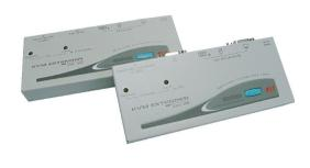
The KVM Extender consists of a Computer Unit and a Station Unit that enables you to locate a keyboard/monitor/mouse setup up to 150 meters away from a computer or KVM switch using an inexpensive Category 5 UTP (unshielded twisted pair) cable. This provides a convenient way to remotely access a computer located in a secure or not easily accessible environment.
