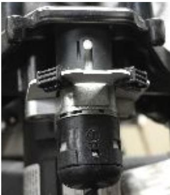
15. Reinstall ignition using provided M8 Bolts
