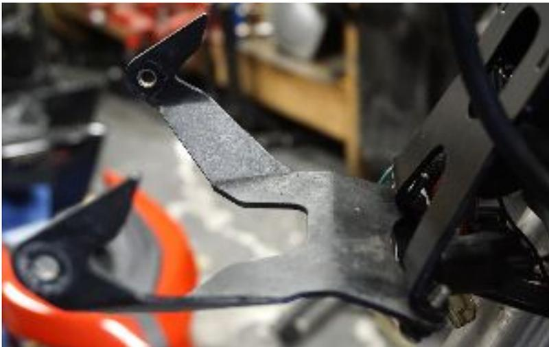
9. Insert the longer M5 bolts through the the underside.
