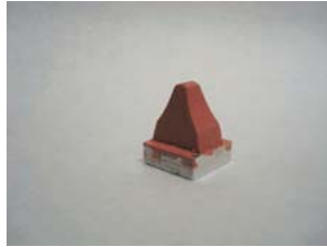
N2 - Overall Height Incl. Base Shown: .96in length at base: .442in Width at base: .96 in Base Shown: (aluminum) .25in x.74 x.74in
