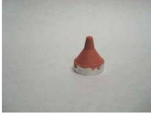
N1 - Overall Height Incl. Base Shown: .87 in. Dia at base: .772in Base Shown: (aluminum) .25in
