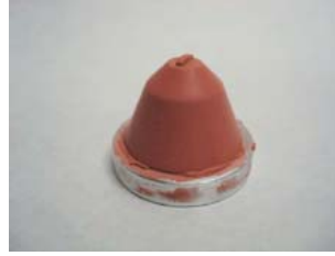
N3 - Overall Height Incl. Base Shown: 1.06 in. Dia at base: 1.3 in Base Shown: (aluminum) .25in
