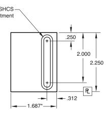
Note: The width of the Actuation Block is smaller by 1/16" to allow for clearance if the CounterView Block is recessed into the mold.
