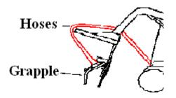
4. Attach one side of both top and bottom Hydraulic Hoses to Cylinder using thread tape(not provided) to prevent leakage.
