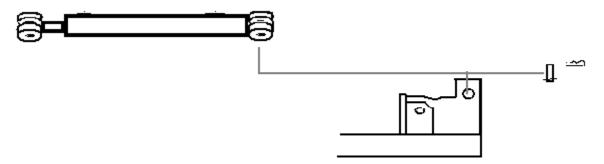
8. Remove key and pin from Cylinder Arm. Extend cylinder or lift arm to match 1 inch hole in Upper Cylinder Mount with Cylinder Arm. Replace pin and key.
