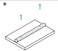
Attach 1 handle centered to the outside of each short box side using 2 screws each. Make sure they slope downward away from the top of the box.
