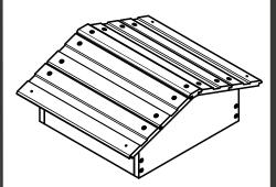
To attach the bottom lower shingles, slide the foot edge under the roof side of the attached shingles. Use the pre-drilled holes to attach the last two shingles.
