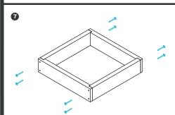
Screw together 2 long quilt sides to the 2 short quilt sides using 8 screws (2 per corner).
