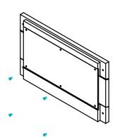
Lay the window rails face down, grooved side up and the plexi glass down into the window rails, lining up the edges so there is a 1/16" gap between them (this allows for wood expansion). Place all 6 selftapping screws in each pre-drilled hole and screw them in.
