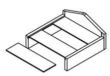
Slide the roof insert panels into the groove. Turn the pieces vertically to slide the insert down into grooves if having difficulty.
