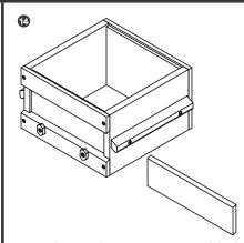
Once these pieces are assembled, flip the window over and slide the window cover in place. There should be no gaps between any of these pieces. This ensures light will not enter the hive once the window is secured.
