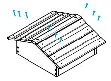
Once this is lined up, attach one shingle at a time with the pre-drilled holes. Fit the ridge cap on the flat surfaces of the peaked roof ends. The ridge cap fits neatly in between the top shingles. If there are gaps, realign the shingles to minimize. 6
