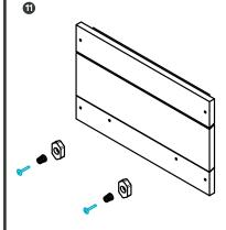
Locate the pre-drilled holes for the walnut latches on the bottom window rail. Insert the springs into the hole on the latches, then insert the spring. Insert screws into the springs. Screw them into place. If these latches are difficult to turn once attached, loosen the screws gently by a couple of turns.
