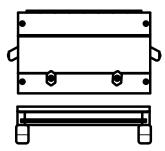
Evenly space 8 top bars into each box. Place screened floor on top of feet and then attach feet using 2 3" screws on each side through the pre-drilled holes in the floor.
