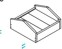
Attach the second peaked roof end to the open end of the side rails. The roof insert should still fit neatly into the peaked roof. Use your drill to secure peaked roof side to side rails.
