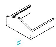
Attach the two roof side rails to one peaked roof end. If you have a clamp, use it to attach these pieces together. Make sure the grooves on all three pieces are aligned. Use a screwdriver or a hand drill to screw the pieces into place.
