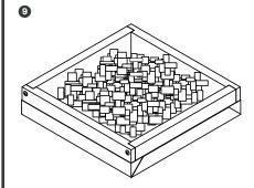
completed, fill Once with wood shavings or some other absorbent, organic material. Hold on to the small canvas. After you assemble the boxes it will lay freely between the quilt box and the top bars of the top box.
