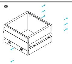
Screw together 1 window side and 1 long box end to 2 short box sides using 12 screws (6 screws per long box end, 4 screws per window side). The box sides need to be flush with the bottom and top rail and should be secured on before the plexi window. Do this for both boxes.
