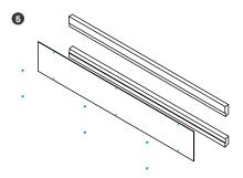
To set the Lexan inside the window side, you will need to bend it a little to fit into end slot and allow enough room for the window to lay flat.
