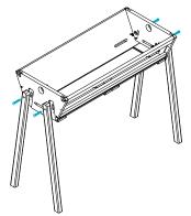
Attach washer from the inside and use wing nut to tighten up. Don't over do it! Secure tightening comes later so don't go nuts... or bolts! Repeat process for remaining 3 legs.
