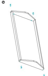
Stand the roof sides up and attach the gabled ends.
