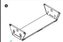
Attach the short ends to the bottom by setting the solid bottom board on a flat surface. At the edge of a table or surface, line up one of the short sides to the board's short end (this makes for easy drilling) and attach. On the other side, do the same.
