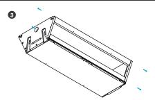
To construct and attach the window side: attach top rail (F1) on the window side to the two short ends with notch side in. Turn hive back over so bottom board is down and hive is right side up. Attach the bottom rail of the window side.
