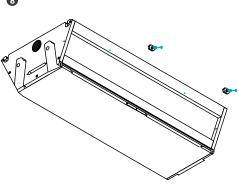
Attach latches for the window using predrilled holes in window top rail.
