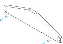
Gather the white nylon bushings. Put 1" screws into nylon bushings into the inside of gabled roof ends, and place into marked indents.
