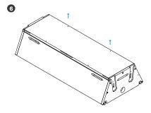
To secure the bottom, flip the hive back over and screw in the last 2 screws thus securing bottom to sides.
