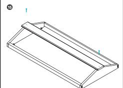
Find the ridge cap (center part of the roof), center it by length and width down the middle. It should overhang on either end about ½" (loose).
