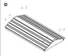
Place top shingles up under ridge cap until they fit with no gap. Locate predrilled holes and attach using 1 long (P) screw on each end of the shingle. Place bottom shingle up under top shingle so they overlap. Tighten ridge cap screws all the way.
