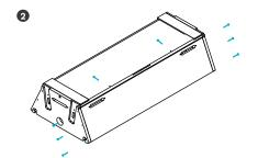
Now to attach the entrance side: flip the hive upside down, attaching the long entrance side to the side ends, making sure no gaps appear.
