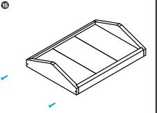
Attach the second peaked roof end to the other ends of the roof side rails. The roof insert should fit neatly into the peaked roof end's groove as well. Use your screwdriver to screw pieces into place. Use clamps on either peaked end to hold the pieces together easily.
