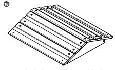
To attach the bottom lower shingles, slide the foot edge under the roof side of the attached shingles. Use the pre-drilled holes to attach the last two shingles.
