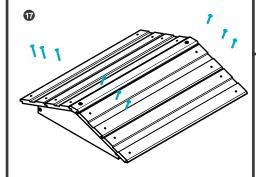
Once this is lined up, attach one shingle at a time with the pre-drilled holes. Fit the ridge cap on the flat surfaces of the peaked roof ends. The ridge cap fits neatly in between the top shingles. If there are gaps, realign the shingles to minimize.
