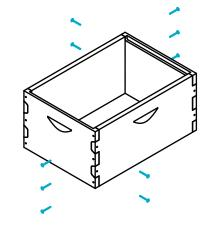
Screw the panels together (5 screws per corner) via the pre-drilled holes. Check to make sure the corners are at 90° angles as you assemble.
