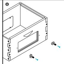
Insert 1" screws into narrow ends of springs and then use to attach latches to window box side.
