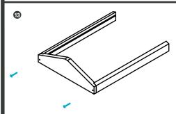
Attach the two roof side rails to one peaked roof end. Make sure the grooves on all three pieces are aligned. Use a screwdriver or a hand drill to screw the pieces into place.
