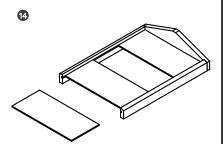
Slide the roof insert panels into the groove. Turn the pieces vertically to slide the insert down into grooves if having difficulty.
