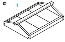
To ensure that all pieces fit together, attach the ridge cap after shingles are attached to the roof. After attaching the top shingles first, you will have a peak and rest under the ridge cap. Line up one shingle with the flat edge on top with the peaked roof end. The ridge cap will not fit if the shingles are not oriented correctly.
