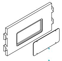
Attach the plexi glass windows to the inside of each window box side.
