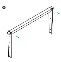
Using 2 long nails, nail one through the side of each end panel into the top bar (on the opposite side of where you nailed in the first 2 nails). This will ensure that the frame doesn't pull apart once its glued in by the bees with propolis.
