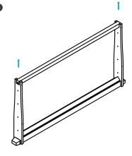
Attach the bottom bar to the frame sides. Using the last two nails, put one nail into the center of the bottom bar, affixing it to the frame sides.
