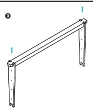
Attach the frame sides to the top. Using 2 long nails, nail one down through each end of the top bar into the end panels on one side.
