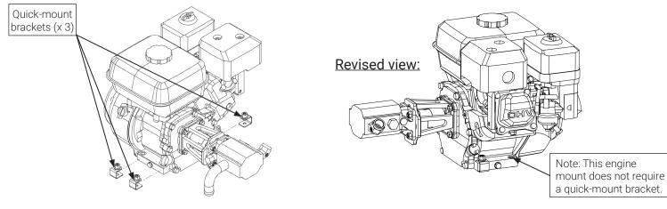
Set one M8 bolt through the bottom of each bracket, through the engine base, and begin threading it into the nut on the top of the quick-mount bracket as shown.
