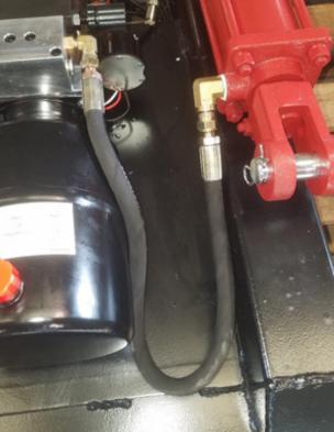
• Verify that the fitting on the valve and cylinder remain tight.
