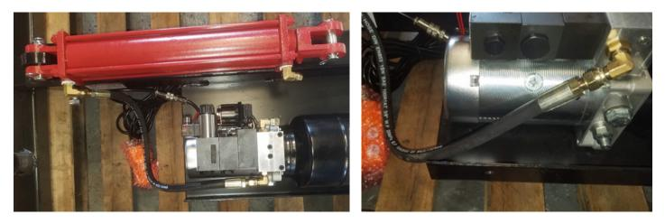
Attach the hydraulic hose (P/N: 31-024) from the hydraulic cylinder's retraction port to the valve of the power unit.
