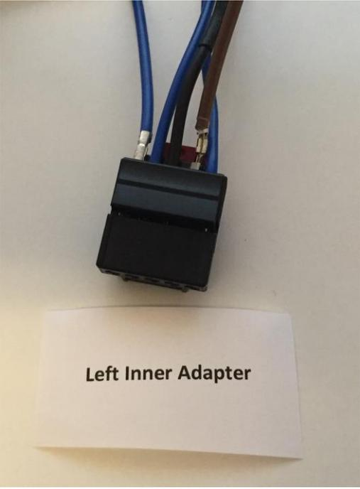
Fig 5, Left Inner Adapter showing all wires installed into it, including the left outer wire.
