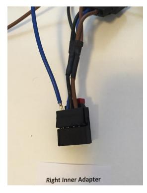
Fig. 7 Right Inner Adapter showing where the blue wire from the outer adapter plugs into Pin 1.
