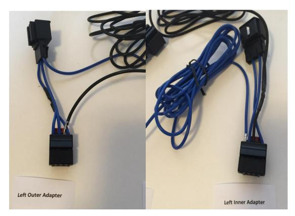
Fig 4. Close Up of where the blue wire plugs into the left inner adapter and the black wire to the left outer adapter to Pin 3.
