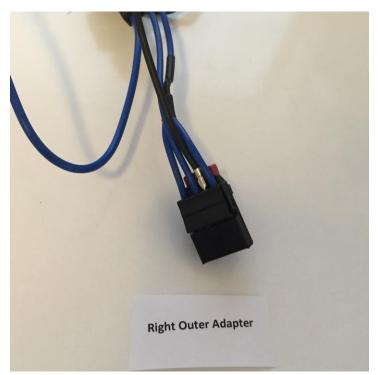
Fig 6. Shows where the black wire from the right inner adapter plugs into the right outer adapter to In 3.
