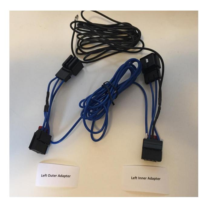
Fig 2. Left Adapters, showing where the wire is ran from the outer adapter to the inner adapter.
