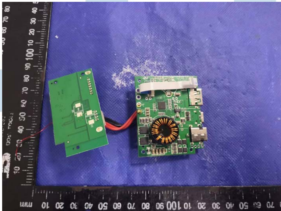
Fig.6- Back view of PCM
