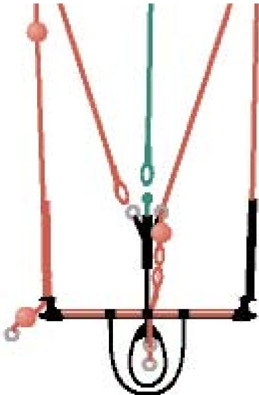
The **SONIC POWERDRIVE CS** allows the rider to interactively change the power of the kite when hooked into the Powerdrive Harness Loop..
