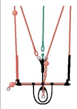
The **SONIC POWERDRIVE CS** allows the rider to interactively change the power of the kite when hooked into the Powerdrive Harness Loop..
