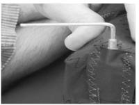
Place the Allen key in the notch located at the trailing edge of the batten pocket. Tension the batten with the Allen key until the wing tip is flat and batten stays in place (i.e. you cannot move it back and forth in the pocket). You do not need positive tension in the wing tip material.
