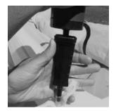
Use one hand to hold the valve steady and the other hand to operate the pump
