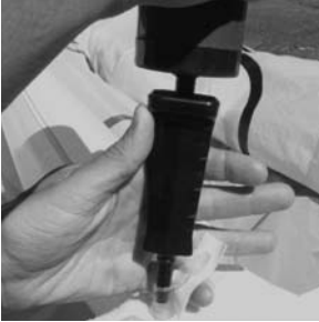
Use one hand to hold the valve steady and the other hand to operate the pump
