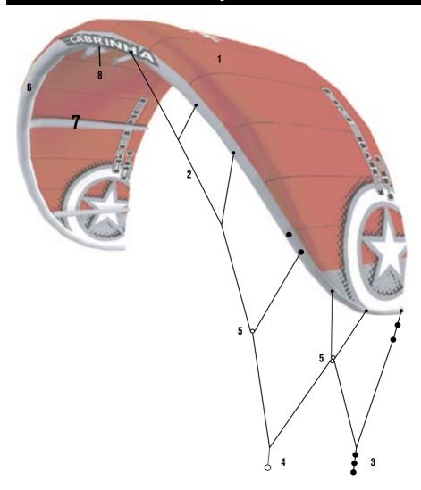
The Omega kite can be switched from a 2:1 bridle configuration to a 1:1 bridle configuration. The 2:1 configuration is for use with a 2:1 [pulley] equipped control system. The 1:1 configuration is for use with a 1:1 [no pulley] control system.
