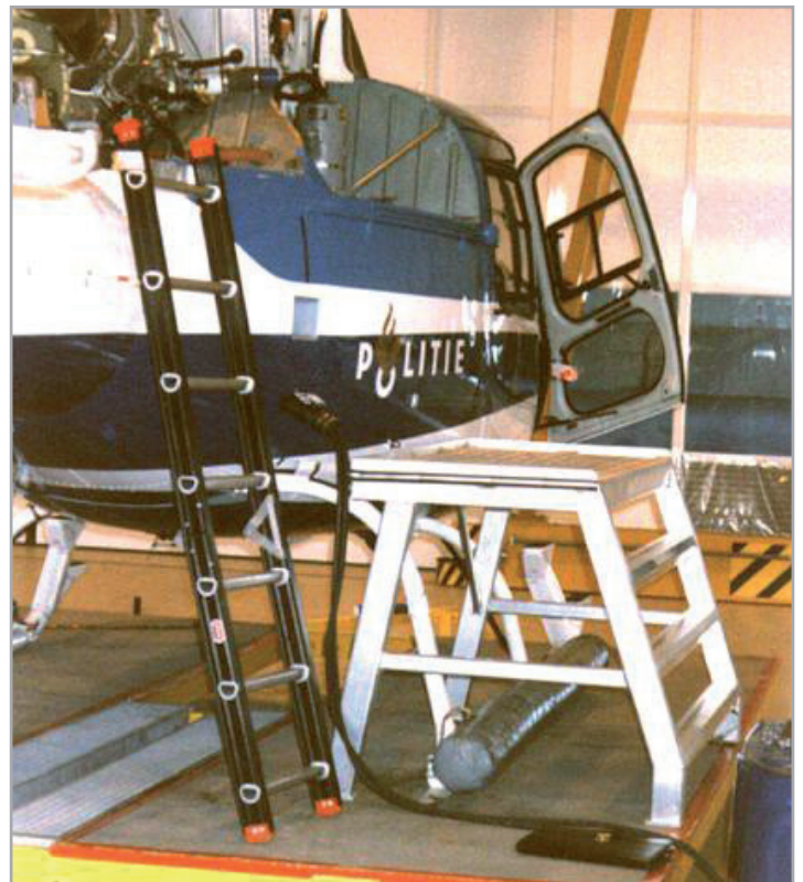
Work platform and access ladder for use by a helicopter
