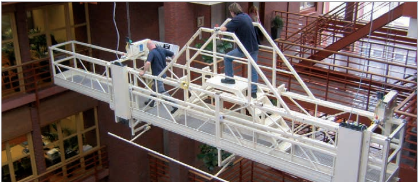
Working platform for roof maintenance window cleaning
