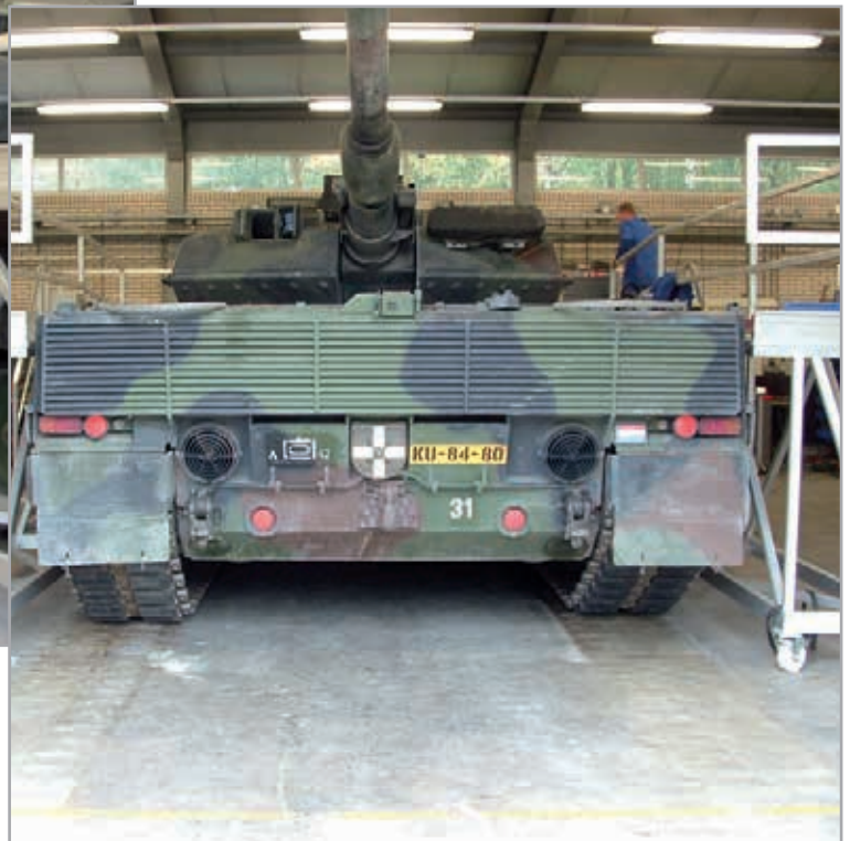
Maintenance platforms Leopard Tank
