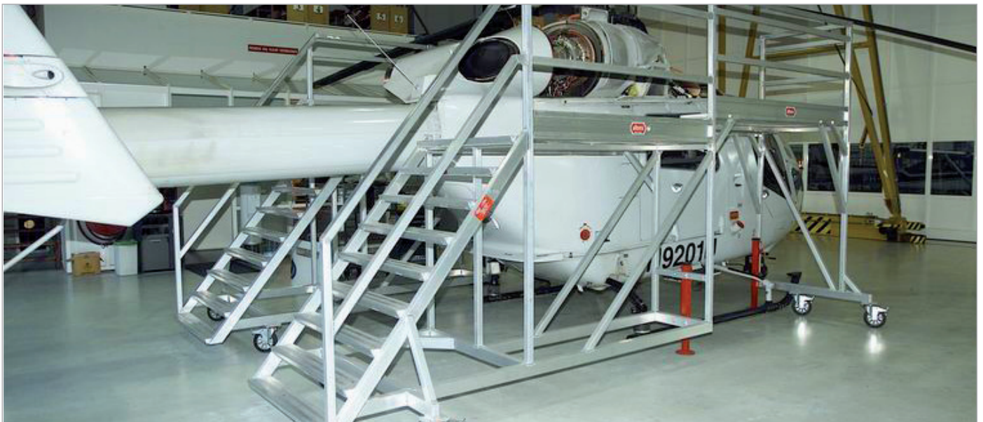
Mobile work platforms around helicopter
