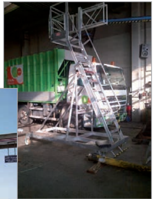
Container stairs/tanker stairs with folding truck fall protection side ways
