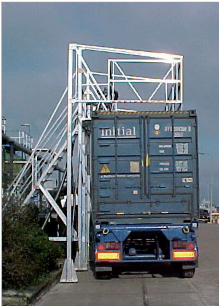
Fall protection system for trucks
