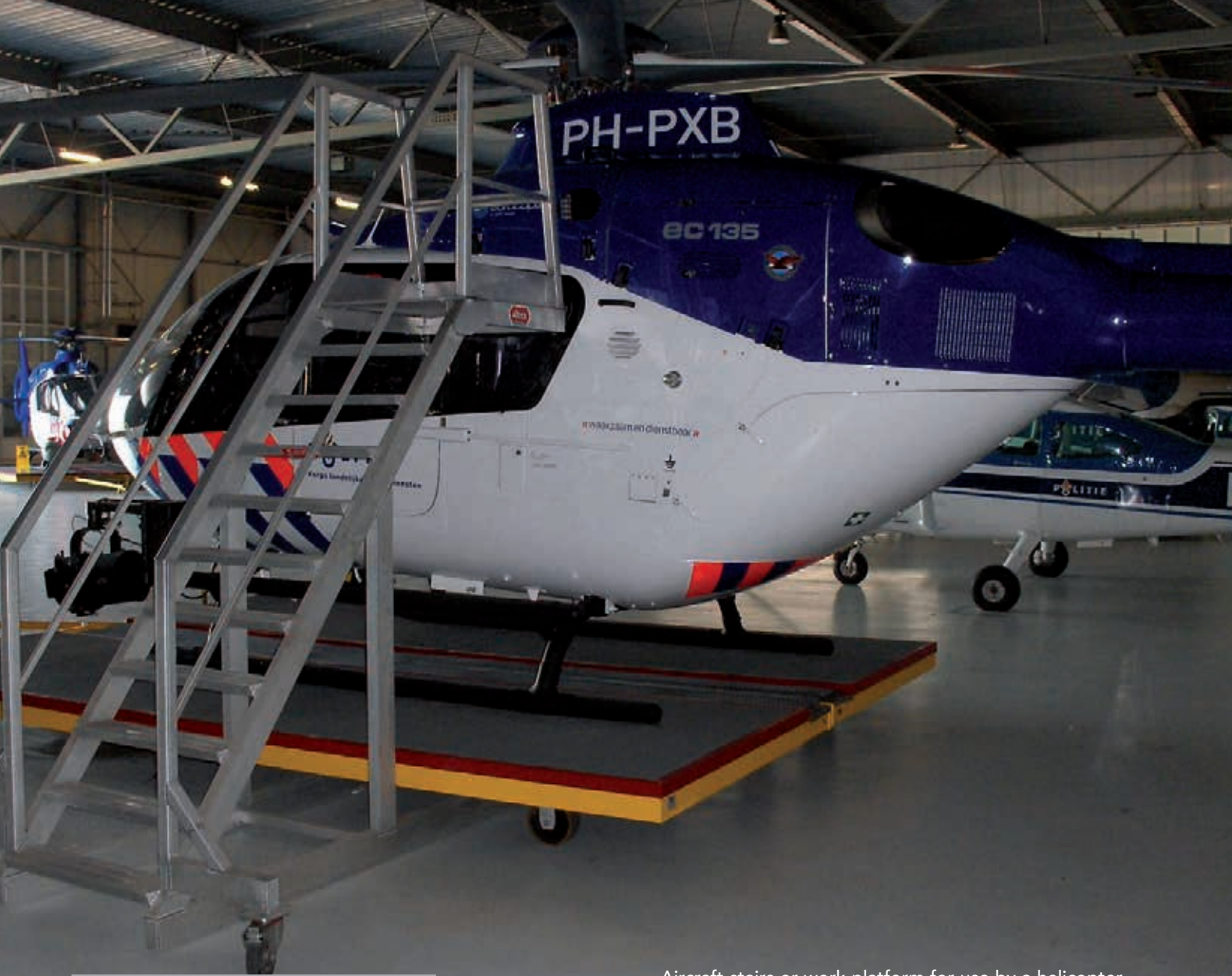
Aircraft stairs or work platform for use by a helicopter
