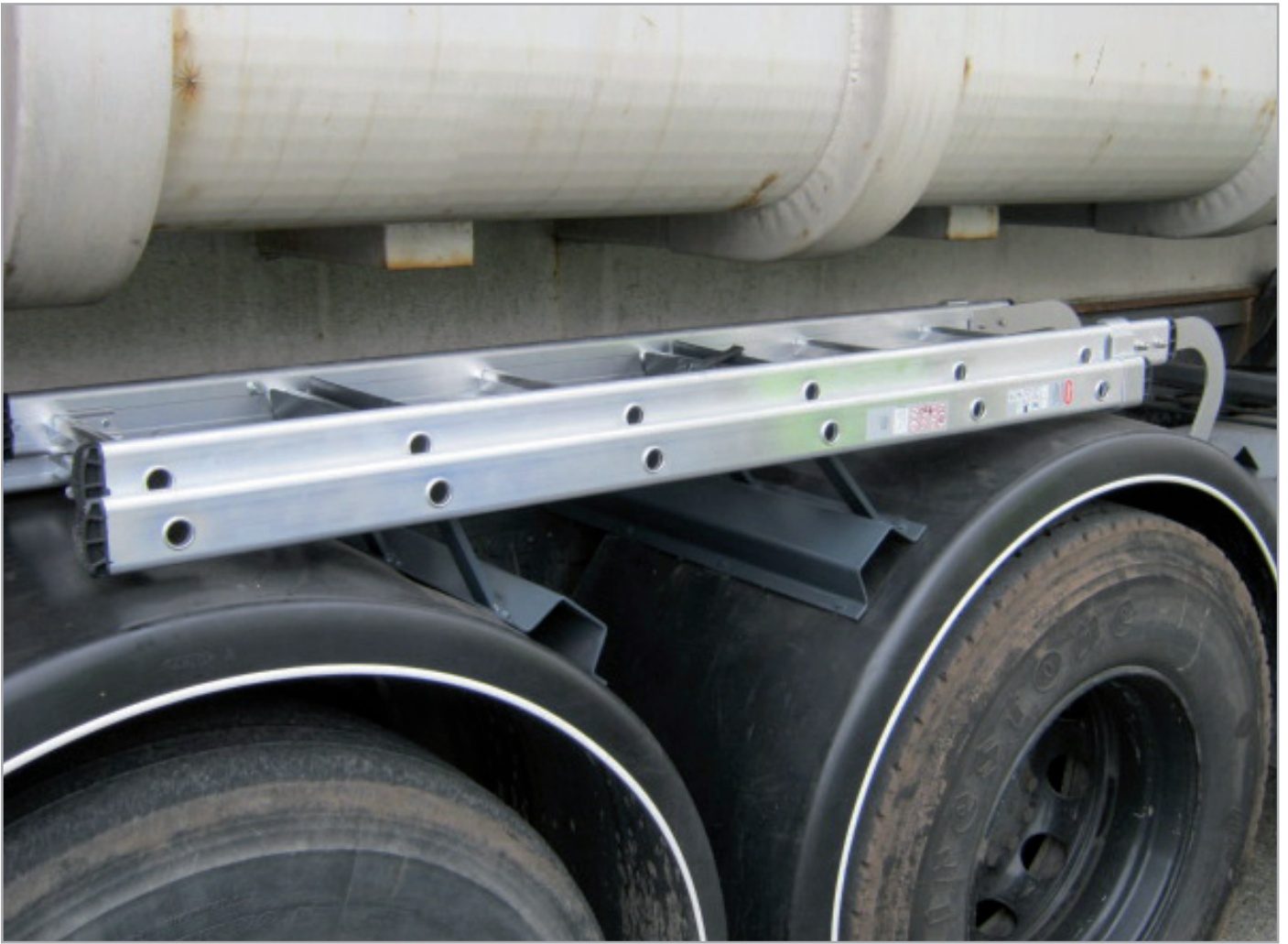
Two-part container ladder fitted with hooks parked horizontally
