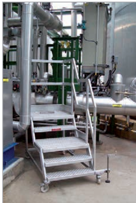
Mobile industrial steps with double platform and brake spindles
