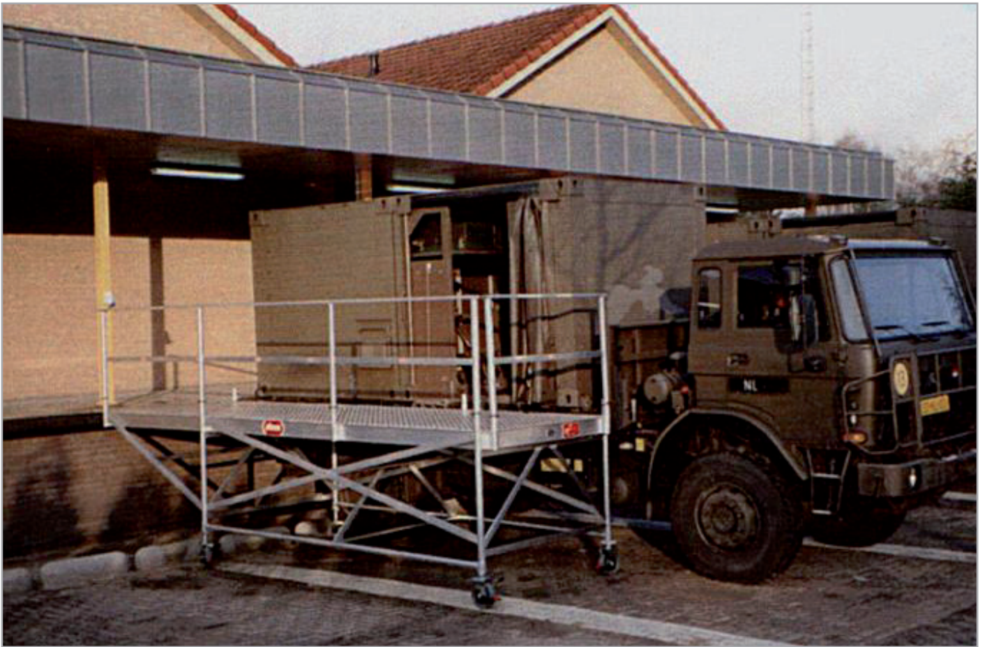
Mobile working platform with cantilever
