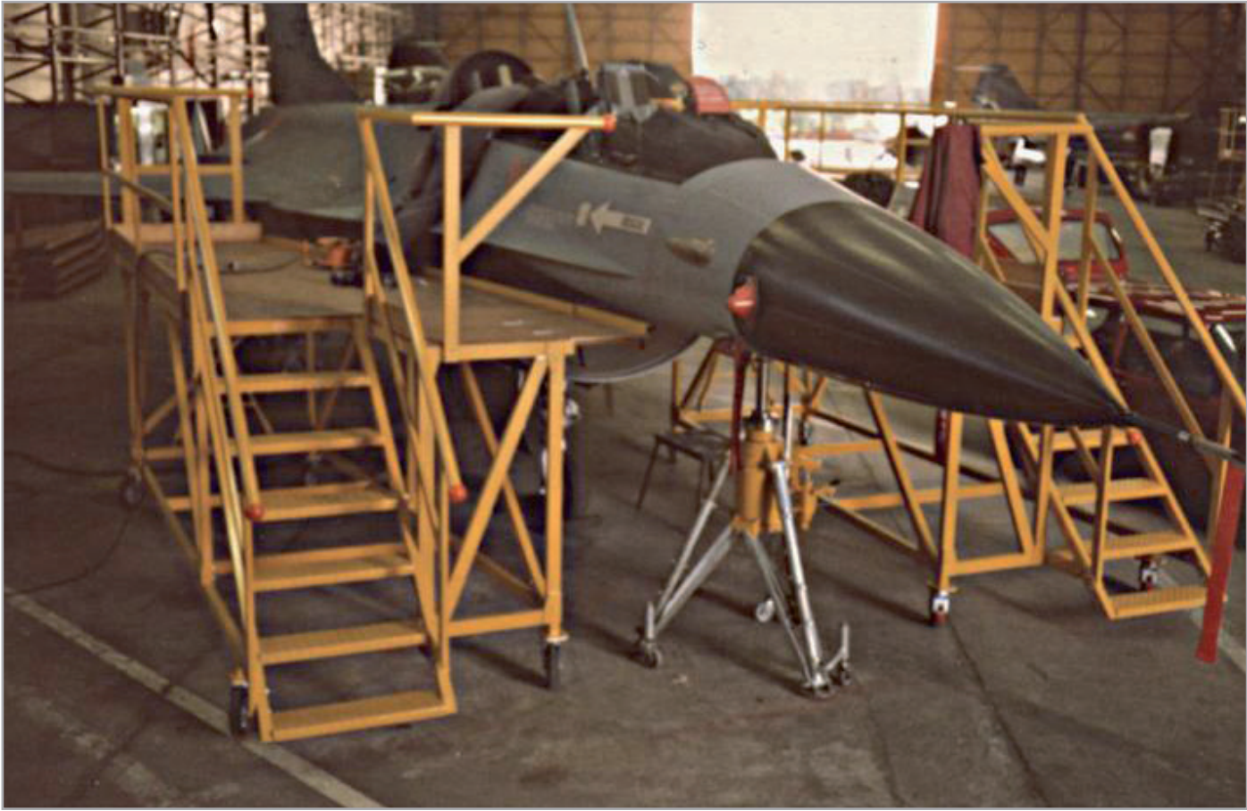
Maintenance work platform Air Force Defence F16 fighter jet
