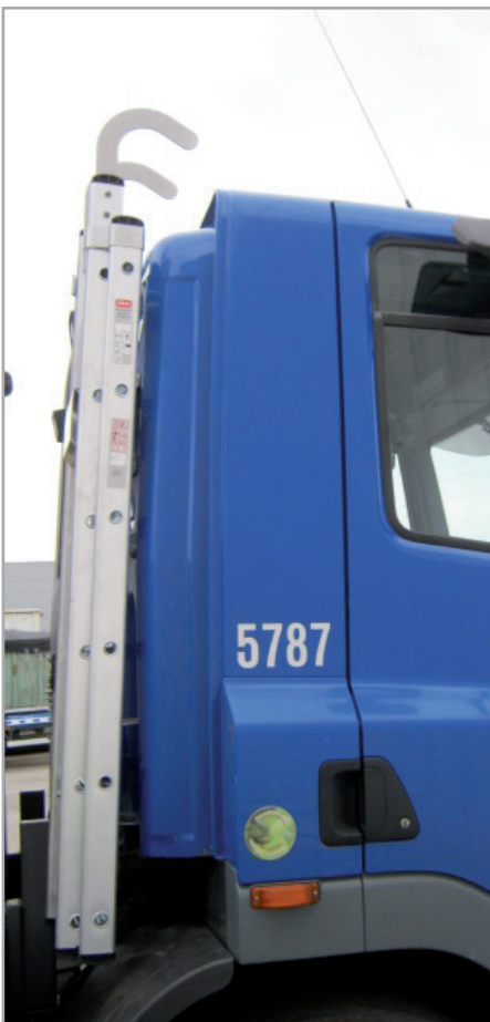
Two-part container ladder fitted with hooks parked vertically
