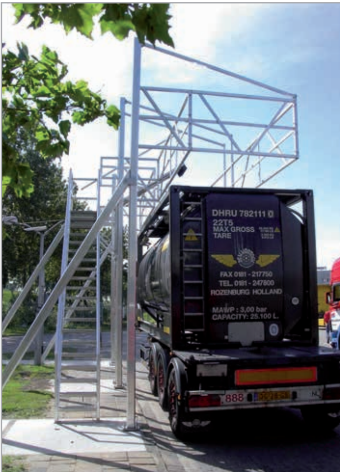
Fall protection system for tankers
