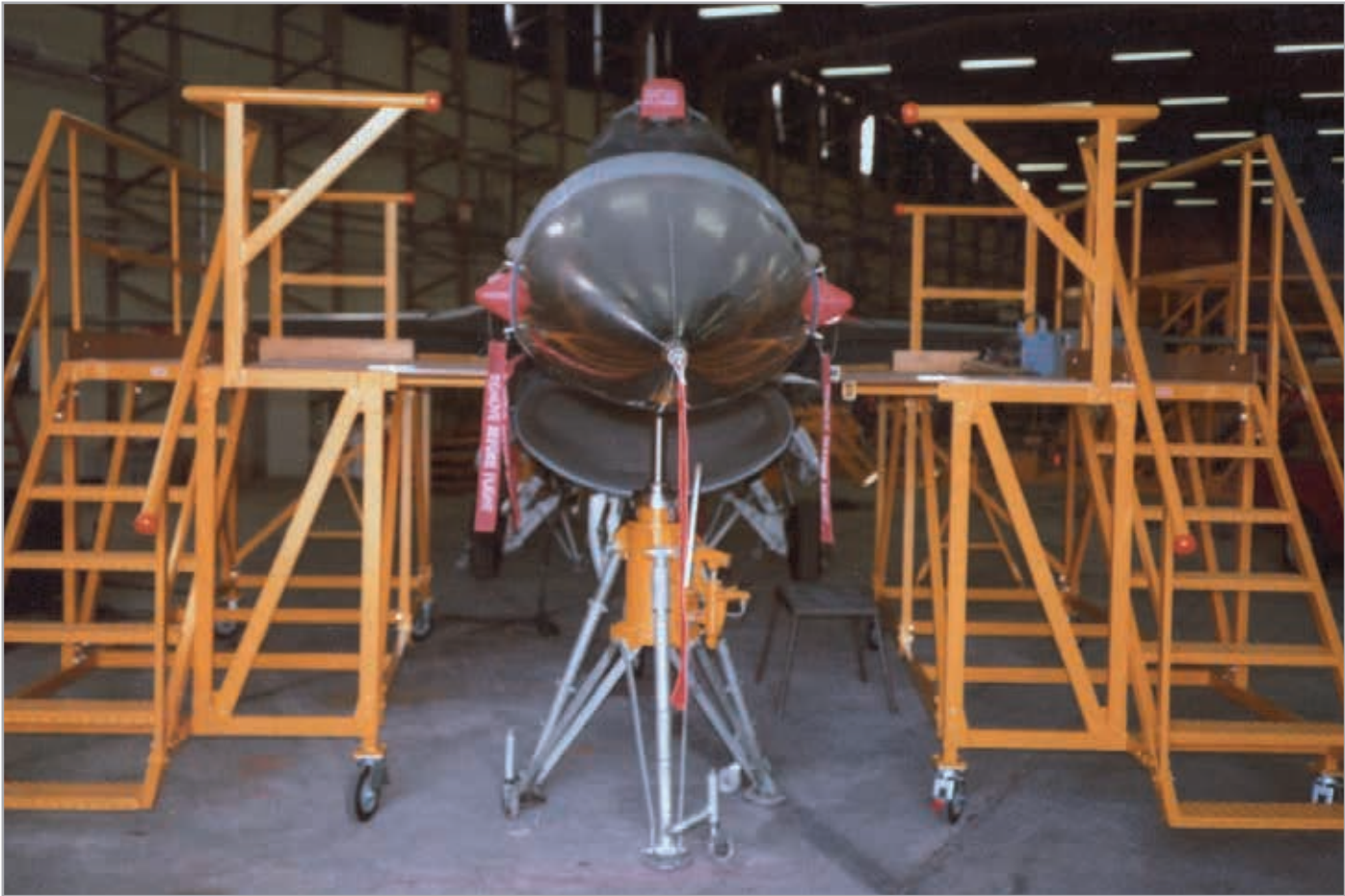
Maintenance platform Air Force Defence F16 fighter jet
