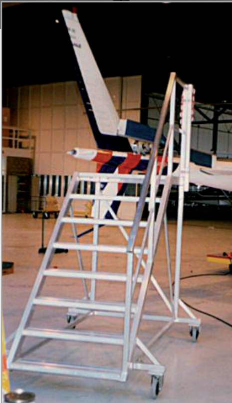
Work platform for use by a helicopter tail rotor
