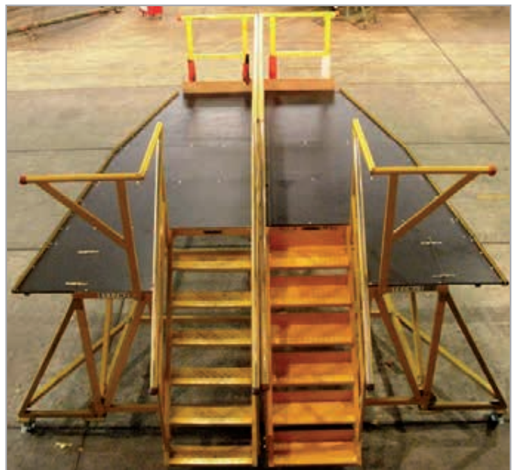
Special maintenance platform
