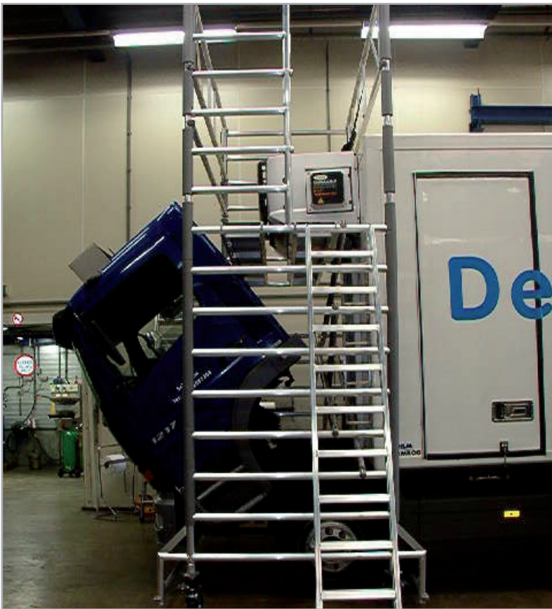
Scaffold for truck cooler unit
