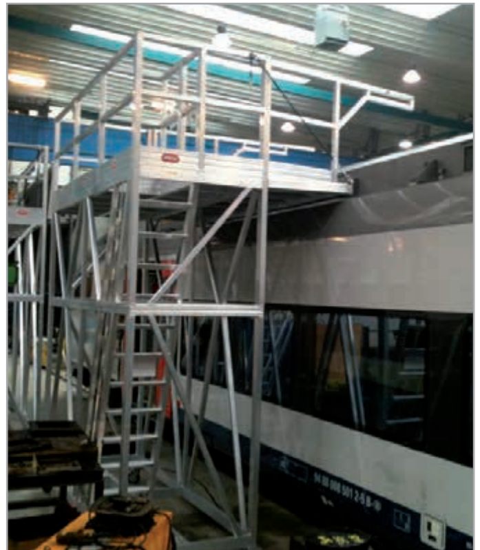
Work platform railway
