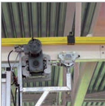
Sideways movable suspension frame maintenance platform
