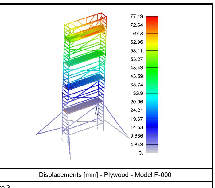
Displacements [mm] - Plywood - Model F-000
