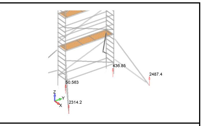
Reaction forces [N] - Plywood - Model F-000
