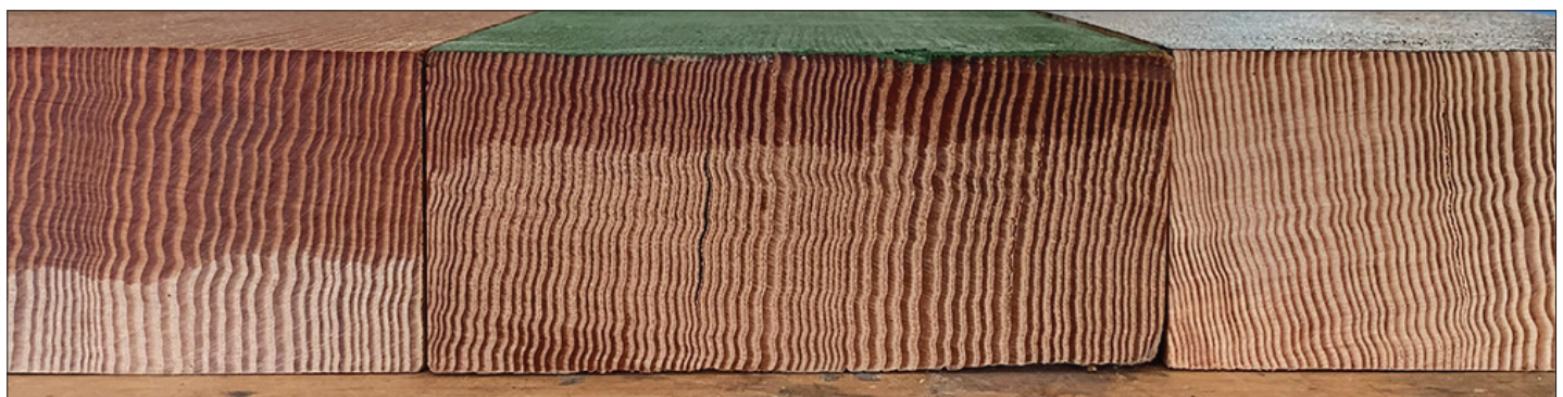
Fig. 4. From left to right, comparison of the absorption of purified raw linseed oil, purified linseed-oil paint, and modern latex paint seen from exposed end grain seven days after application. Raw linseed oil has been absorbed the most deeply; boiled linseed oil used in the linseed-oil paint has absorbed only shallowly. The latex paint is not absorbed at all and remains on the surface, 2020.
