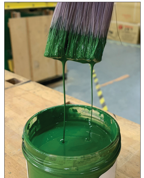
Fig. 9. Linseed-oil paint has an extremely thin consistency and must be applied in thin layers. The amount shown on the brush would cover approximately 4 square feet or more, depending on the condition of the substrate, 2020.
