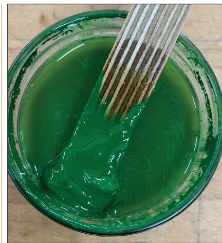
Fig. 2. Linseed-oil paint is made of purified boiled linseed oil and earth pigments, which settle to the bottom as a mass over time and require stirring to evenly disperse the pigment into the paint. Linseed-oil paints also contain traces of manganese to shorten drying time and in some cases, less than 3 percent paraffin to add flexibility, 2020.
