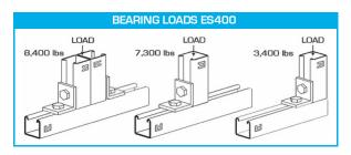
Resistance to Slip: 1,500 lbs. per bolt when 1/2" ES NS channel nuts are used. Pull Out Strength: 2,000 lbs. per bolt when 1/2" ES NS channel nuts are used.
