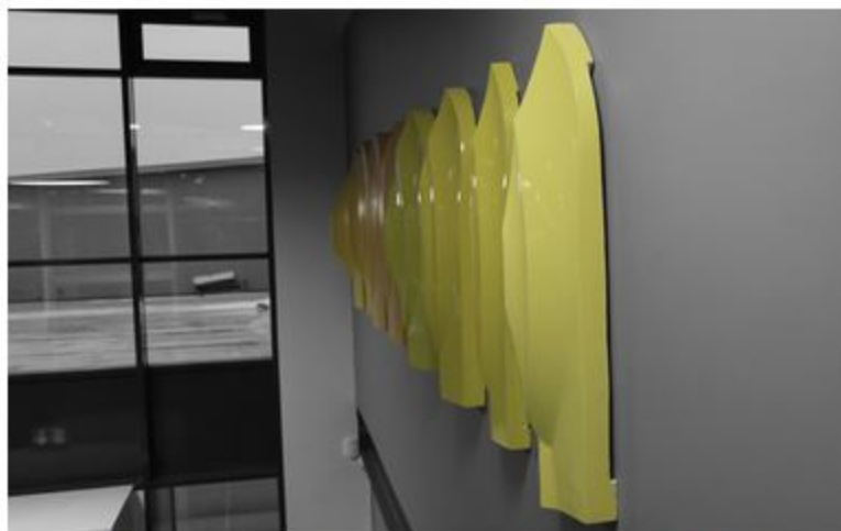
A selection of the models used in tank testing hang on the walls in the office
