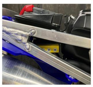
**Step 5:** Secure the 4 way Programming cable and 8 Way Options cable coming from the Vortex ECU with the zip tie provided. **NOTE:** Do not over tighten zip ties on any wiring
