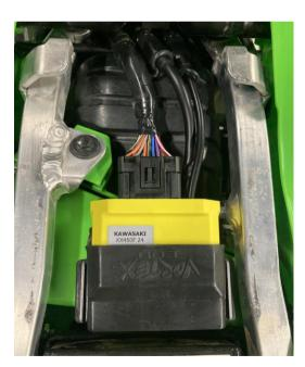
**Step 6:** Carefully plug the 33 Way connector onto the VORTEX ECU and push firmly until the locking tab clicks. Route the black Vortex ECU Programming harness (with rubber cap) and \* way Options Port Connector in front of the ECU towards the fuel tank and lightly zip tie to the main harness. **NOTE:** Do not over tighten zip ties on any wiring
