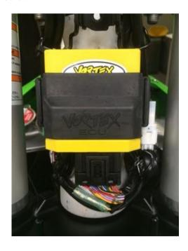
**Step 6:** Carefully plug the 33 Way connector onto the VORTEX ECU and push firmly until the locking tab clicks. Bolt the small bracket and 2 std diagnostic connectors previously removed back into place with the 10mm bolt. Route the black Vortex ECU Programming harness (with rubber cap) in front the ECU and zip tie to the standard diagnostic connectors as per the above picture.
