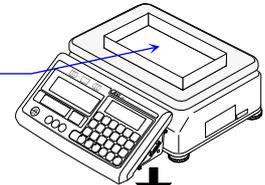
Step 2. Press the **SAMPLE** key. The scale subtracts tare weight (container weight) from weighing value and displays **Add Sample** and **10 pcs** automatically.
