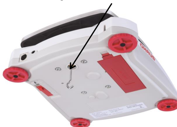
Weigh Below Hook installed
