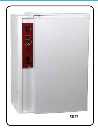
SHEL LAB Refrigerated Incubators (often called B.O.D. Incubators or Low Temperature Incubators) are commonly used for applications such as B.O.D. Determinations, Plant and Insect Studies, Fermentation Studies, and Bacterial Culturing. The SHEL LAB Low Temperature Incubators have a temperature range of 20°C degrees below ambient to 45°C.
