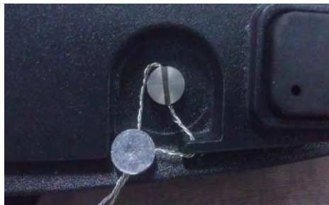
Locked with Wire Seal
