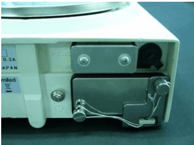
Typical sealing / Scellage typique
