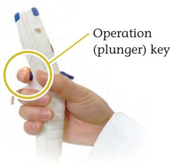
With the MPA series, it is possible to control the plunger by lightly pressing a key with the ball of the forefinger (like pulling a trigger), while maintaining all fingers in a natural, effortless grip. No longer will hours or days of pipetting make you feel any pain in your thumb.\*1
