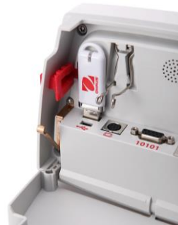
Interface connections on back of Terminal.
