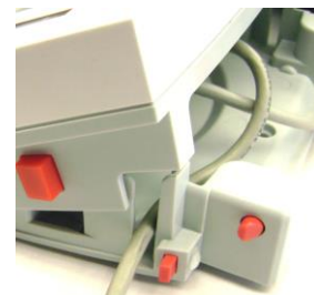
Interface connections on back of Terminal.
