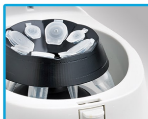
Combination rotor accepts 1.5/2.0ml & 5ml centrifuge tubes
