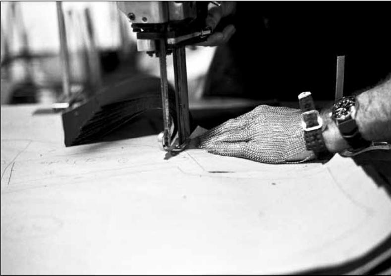
**Fig 8** A worker cuts through many layers of denim, using a paper pattern as a guide. A metal mesh glove is worn to protect the hand. Photograph by Nick Pironio.
