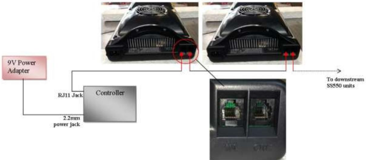
NOTE: If any SS 550 unit in the chain loses power, the communications will not be interrupted to downstream units. This is a unique feature of the SS 550 systems.
