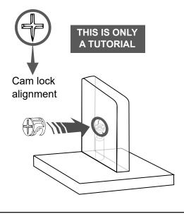
2. Join the other panel (with the big hole) to the panel with the bolt. If it comes with the cam locks already pre-installed, make sure to align them to receive the bolt's head (refer to point 3). There might be a very small gap between the panels which is normal.
