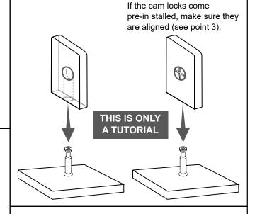
4. Use a Phillips screwdriver to turn the cam lock clockwise. This will lock the panels togheter and also will close any gaps.
