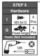
Pay attention to the orientation of the fixed hinges G, and attach them to the side panels 6 and 10 with screws I.
