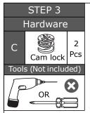
With the pieces placed oriented as shown, ensamble the partition panels 7 and 9 to the shelf 8 with cam locks C as explained in the **TUTORIAL PAGE**.
