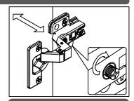
To adjust side-to-side, loosen up or tighten this screw.
