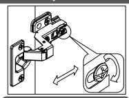
To adjust the depth, loosen up this screw, align, then retighten
