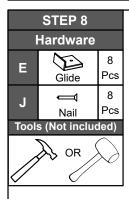
On the indicated profile of the skirting boards 1 and 4 install 2 pieces of the glide feet E using nails J at approximately 2" from each end, then another 2 pieces E in the middle at equidistant length.
