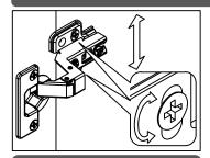
To adjust the height, loosen up these screws, align, then re-tighten
