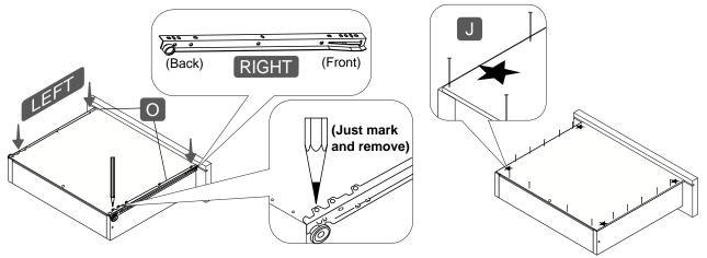
• Assemble the "L" shaped sliders **O** on their respective sides with screws **H**, but please note: The wheels go towards the back of the drawer.
