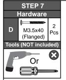
Assemble the lower panel 5 to the middle panel 4 with flanged screws D as shown.
