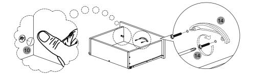
Assemble the handles (14) to the front panels (O) and (P) on both drawers using the screws that come with them. Please note the orientation of the handles. Then cover the cam locks with the plastic caps (10).
