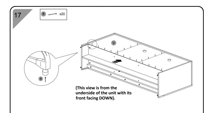
Attach the back panel (V) to the backside of the unit using nails (8) as shown, but please pay attention to the orientation of the cable holes on the panel.
