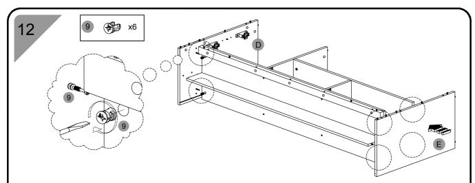
Install and align the cam locks (9) to the bottom panel (B) and middle shelf (C) in the locations shown, and assemble the panel (D) to (B) and panel (E) to (B/C) as explained in page 4.
