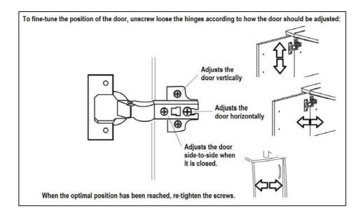
Assemble the Door (N) to the unit by joining the 2 parts of the hinges as shown
