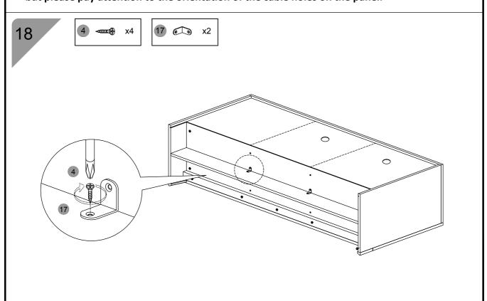
Attach the L bracket (17) to the panels (B) and (H) using screws (4) as shown.
