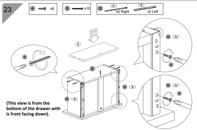
Assemble the back panel (S) to the panels (R/Q) using screws (5) as shown. Then grab the "L" shaped sliders (12) and assemble them to the bottom of the drawers using screws (4) as shown. NOTE: their wheels will be facing towards the back of the drawer. Also make sure the sliders are in contact with the wood on the bottom and the side.
