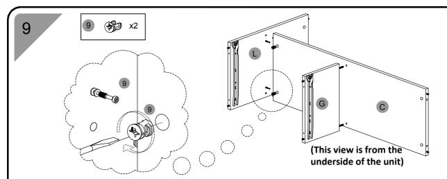
First install and align the cam locks (9) to panel (C), then assemble the panel (L) to (C) as explained in page 4. Finally, join the panel (G) to panel (C) as shown.
