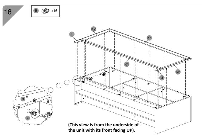
First install and align the cam locks (9) to the panels (A/B/D/E) in the locations shown, then assemble the Top panel (A) as explained in page 4.
