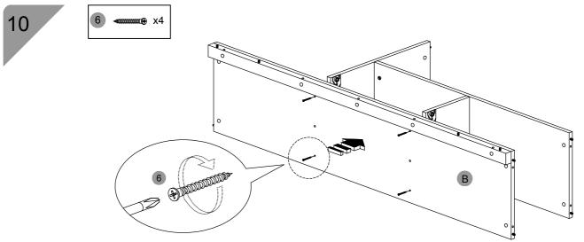
Assemble the Bottom panel (B) to panels (G/L) using screws (6) as shown.
