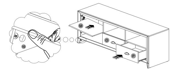
First insert the drawers into the unit, making sure the drawer with front panel (O) goes on the LEFT and the one with panel (P) goes on the RIGHT. Then insert the Shelf panel (M) into the unit. Finally, cover the cam locks that are visible at the front of the unit with the plastic caps (10).
