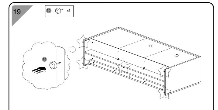
Attach the plastic feet (15) to the panels (D), (E) and (H) as shown.
