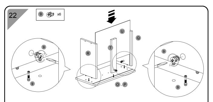
First install and align the cam locks (9) into the corresponding holes on panels (R), (T) and (Q) as explained in page 4. Then Assemble those panels to the Front panels (O) and (P) respectively as explained in page 4. Finally, slide the bottom panels (U) thru the grooves of panels (O/P/R/Q).
