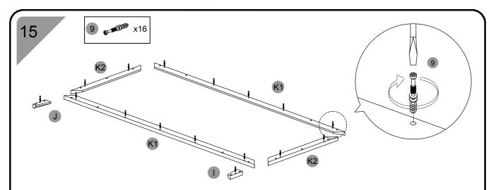
Attach the cam bolts (9) to the panels (I), (K1) and (K2) in the corresponding holes as shown, but make sure to use the correct holes as some are intended for other kind of hardware in subsequent steps.
