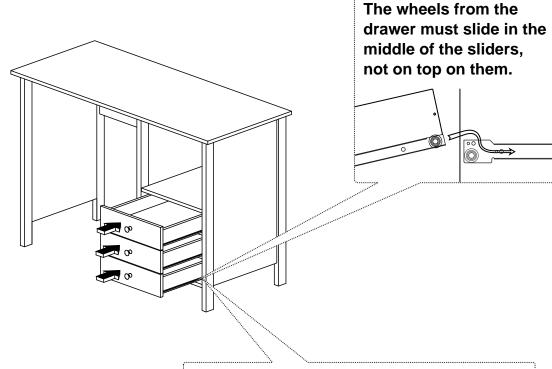
If the drawers stop or feel like hitting something, tighten all the screws as flushed as possible so the heads don't interfere with the rollers.
