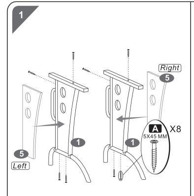
Use Screws (A) to assemble the Side Panels (5) to the Main Structures (1).
