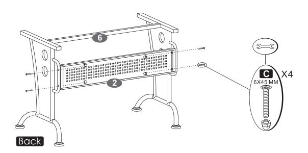
■ Use Screws (C) to assemble the Back Panel (2) between the Main Structures (1).
