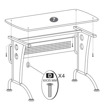
■ Use Screws (D) to assemble the Main Panel (7) to the Main Structures (1).
