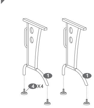
■ Insert the Studs (4) to the Main Structures (1).
