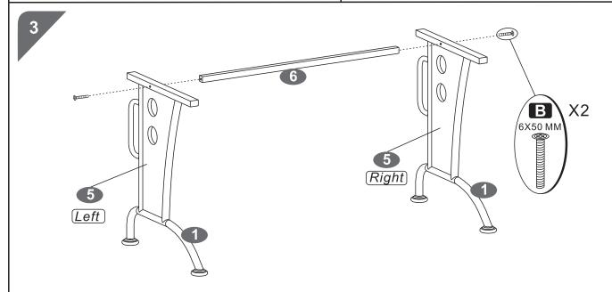
• Use Screws (B) to assemble the Horizontal Tube (6) between the Main Structures (1).
