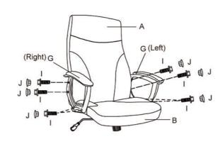
Place the seat over the base,making sure the tip of the gas lift enters into the hole of the mechanism.
